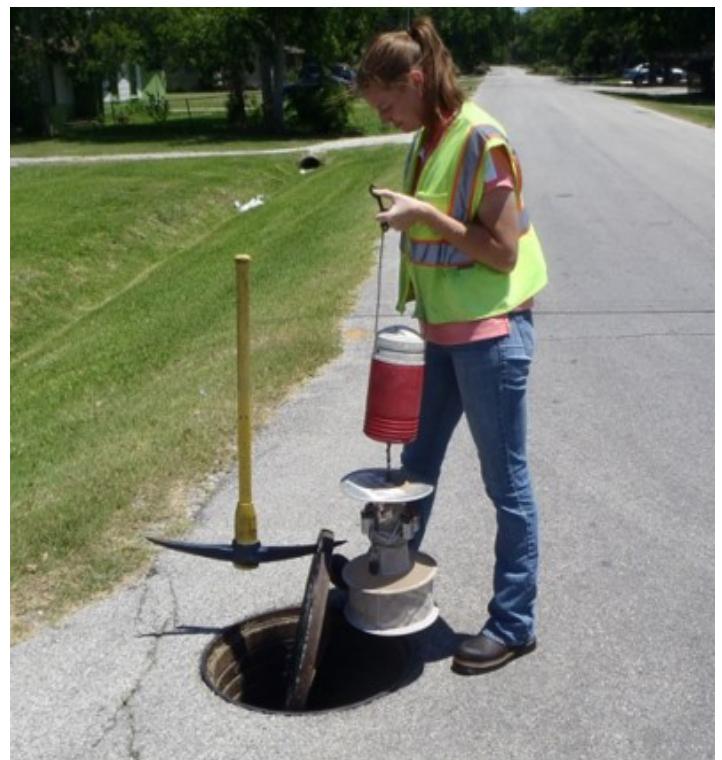
Figure 6. CDC Light Trap baited with carbon dioxide being placed into sewer
