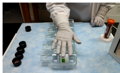
Figure 8. Rolling bottles to evaporate liquid.
