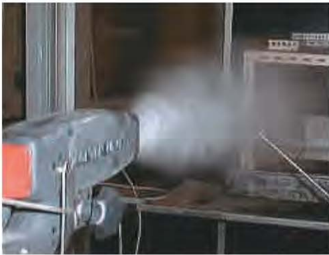
Figure 1: Cold fog from the Starlet directed at laser beam with the DC-III sensor in spray cloud.
