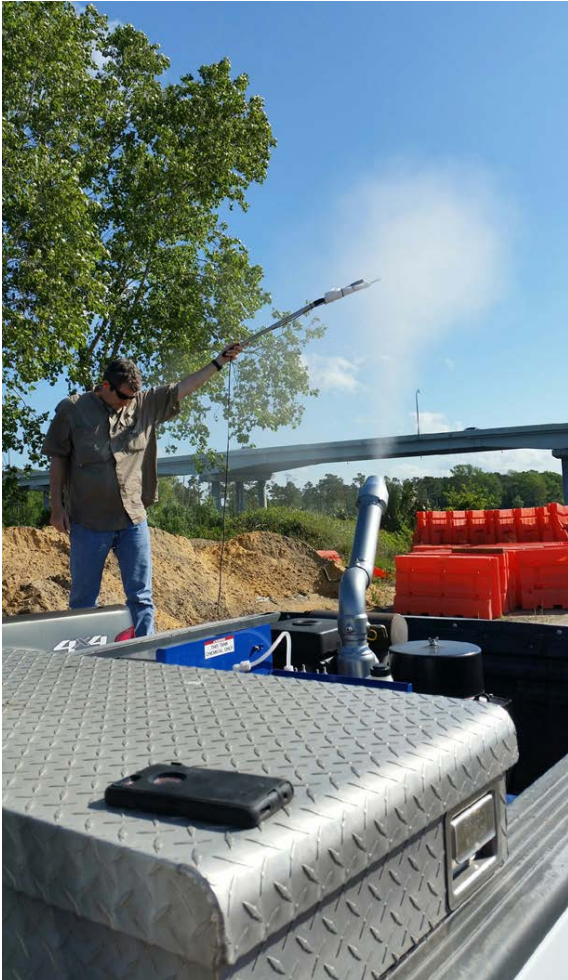
Trey English and Larry Heller with Adapco measuring droplet size from ULV equipment
