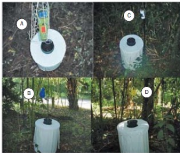
Figure 3. Photos of each of the 4 test items suspended over the BGS Sentinel trap using rope and shepherd hooks: A - ThermaCELL Mosquito Repellent B - OFF! Clip On C - Lentek Bite Shield D - Bug Button Mosquito Eliminator
